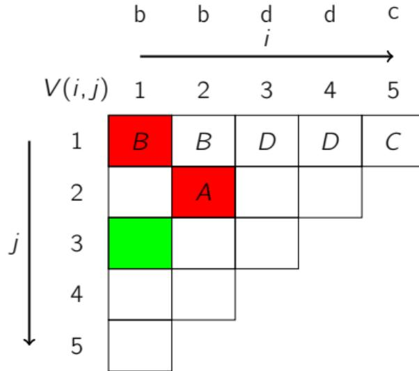
3-fache Schleife:  $j = 3, i = 1, k = 1: V(1, 3) = V(1, 3) \cup \left\{ A \mid \begin{array}{l} A \rightarrow BC, \\ B \in V(1, 1), \\ C \in V(2, 2) \end{array} \right\}$
