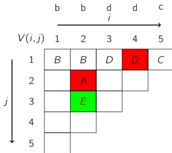
3-fache Schleife:  $j = 3, i = 2, k = 2: V(2, 3) = V(2, 3) \cup \left\{ A \left| \begin{array}{l} A \rightarrow BC, \\ B \in V(2, 2), \\ C \in V(4, 1) \end{array} \right. \right\}$
